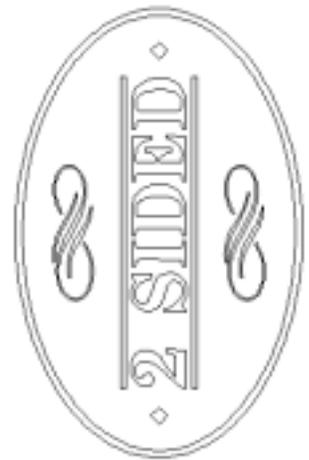
**STEP 2.** Select the entire job and do an Absolute Move so that the lower left corner of the sign lines up with the X= 0.0 & Y= 0.0 coordinates on the Composer screen.
