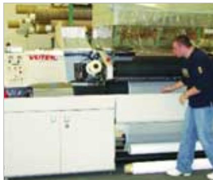
Northstar's workhorse printer is the VUTEk UltraVu 5300, used to print all of its building-sized graphics, fleet graphics, and much of its trade show work.
