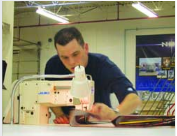
Finishing banners sometimes requires the use of a heavy duty Juki sewing machine.
