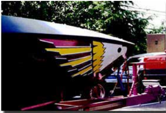
The graphics on this 40-ft offshore race boat are a combination of EDGE and straight cut vinyl work. The Eagle is 12 feet long, and its head is about 4 1/2 feet high. A checkered flag design that fades in and out from black to white covers most of the boat's side.
