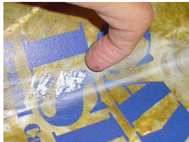
Traditional free-radical inks come off easily when scratched.
