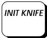
The **INIT KNIFE** key is for initializing the swivel knife so that it is in a known position (blade faces 0°). We recommend that you initialize the swivel knife before every job, if you have changed material, or after the tool has been loaded. It is not necessary to initialize the tangential knife.
