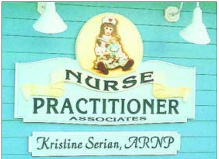
This panel is 1 1/2" HDU cut to shape, with hand carved incised lettering. The cameo is airbrushed, clear coated and applied separately; ANP gooseneck lighting.
