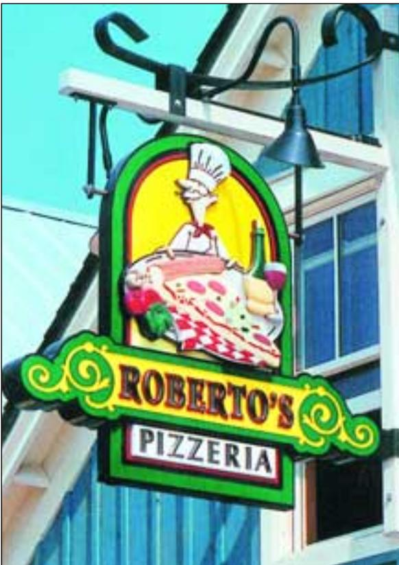
Roberto's Pizzeria sign is made with HDU, laminated with West System Epoxy and hand carved. Letters are prismatic cut 3/4" HDU on 1/4" PVC. The custom welded frame is mounted to white-washed poplar and externally lit.
