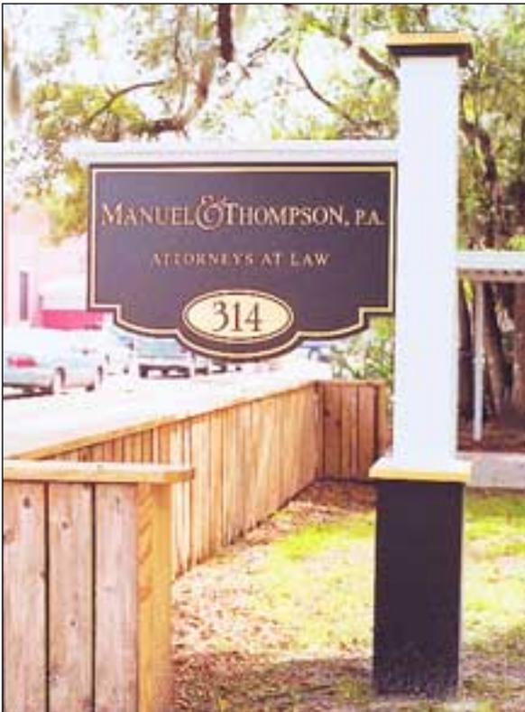
This post blade sign is made of 3/4" and 1/2" sheet PVC panels, V-cut and hot folded to fabricate the post system. The upper swing arm is 1/2" PVC V-cut and folded and attached with a custom routed insert into the upright post. The 1/2" PVC profile-cut blank is used as a 90-degree fill-in; painted automotive black with 23-karat gold leaf accents and post caps.
