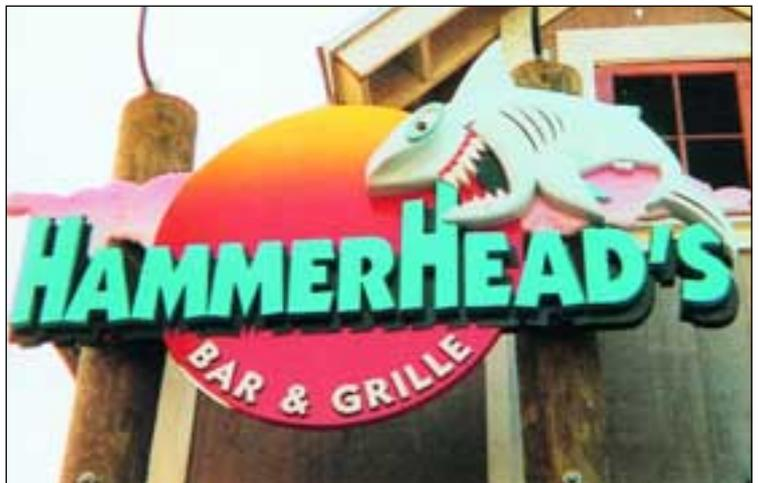
This bar & grill sign is another Baytown Wharf project, measuring 130" x 65" and is mounted to existing wharf timbers. Made of multiple pieces of 3/4" MDO backer board with 1/4" PVC "HammerHead" letters painted black. The blue letters on top are 1 1/2" flat-cut HDU and the sun is 1/2" HDU. The shark is 1 1/2" HDU cut to shape, stack laminated and then hand carved.
